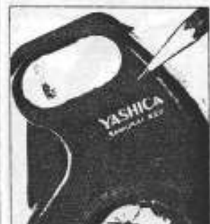
LED located below flash unit on front provides visual only indication of electronic self-timer.
