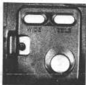
Power zooming and shutter release buttons are grouped in uncluttered area at top of camera's right side.
