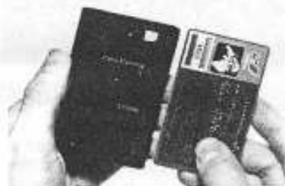
Don't leave home without it: Lemix Card Camera (collapsed) has height and width of a credit card. Depth? A watch-pocketable one-half inch.
