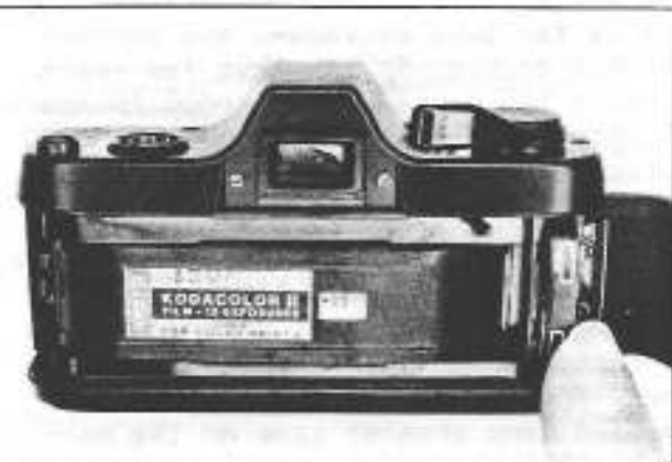
Batteries (two S-76s) are held in tiny tray that nests in compartment near the back's doorhinge.
