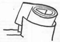
To put the roll of film in the supply side cassette, tilt it at an angle and use the leader to find the light trap slit.
