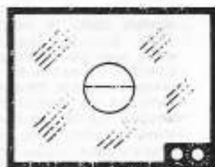
Viewfinder is bright corner to corner with large, clear, split-image rangefinder in center. LEDs in lower right provide green go-ahead signal, and yellow light to indicate shutter speed is too slow for hand-held exposures without flash.
